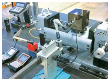
Measuring a T-type rotary table with a cube
