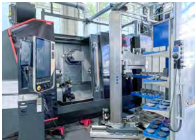
With workpiece pool for unmanned production
