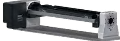
EA-520 rotoFIX with clamping yoke pL 1000 mm and mounted TRIAG rails
