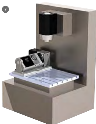
4 th + 5 th axis, 2-spindle, Y-mounting (crosswise)
