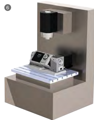
4 th + 5 th axis, 1-spindle, X-mounting (lengthwise)
