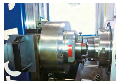
Measuring the indexing accuracy – fully automatically
