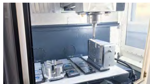
Application of a 4 th axis on a 3-axis machining center
