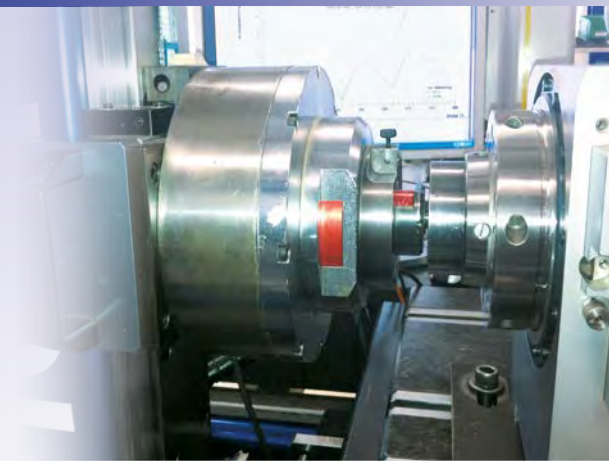
Fully automated measuring system for indexing accuracy measurement
