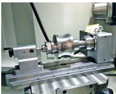
EA-510 longFLEX – Milling/boring on horizontal center – Mechanics
